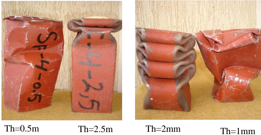
Figure (10) Effect of tube thickness on the collapse modes
